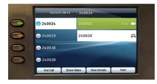
To connect the second call and put the first call on hold automatically, press the flashing amber line button .
